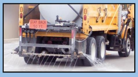
components of **InfernalMelt R** are responsible for two important aspects of the product; 1.) Due to the high levels of sugars in the product we get significant corrosion inhibition. 2.) The sugars, along with the long molecular chains of the polymers give it a tenacious bond to the pavement. This residual effect equates to the product remaining on the pavement longer which ultimately means less is needed for the same level of service.
